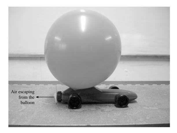
When the air in the inflated balloon is released, the car starts to move forwards.
